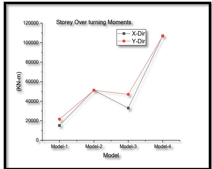
Chart 5: Max storey over turning Moments for irregular building with shear wall(Model 4)
