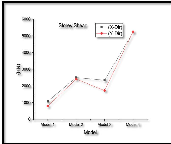
Chart 3: Max storey Shear for irregular building with shear wall(Model 4)
