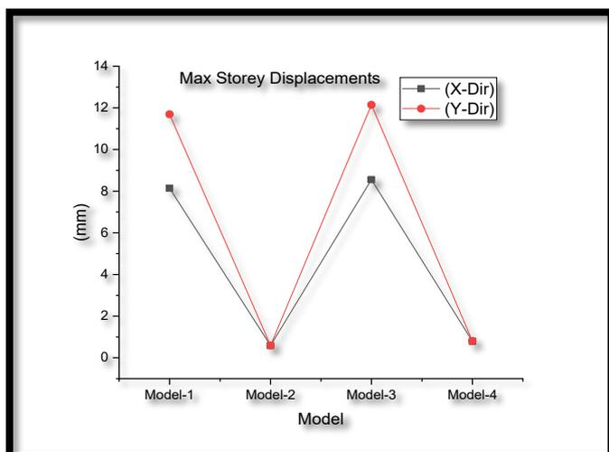
Chart 1: Max storey displacement for irregular building without shear wall(Model 3)
