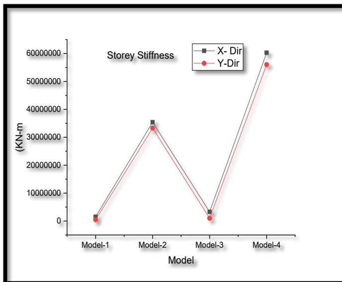
Chart 4: Max storey Stiffness for irregular building with shear wall(Model 4)
