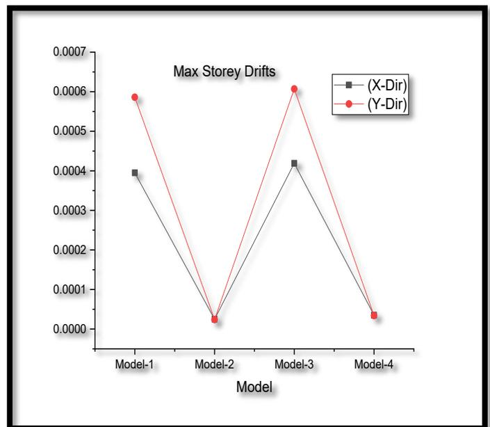
Chart 2: Max storey drift for irregular building without shear wall(Model 3)
